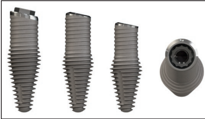
Fig 8 From left to right: Inversa Co-Axis hybrid implants were used with a "body shift" in diameter of 1.0 to 1.5 mm (ie, 5.0-mm tapered apical portion and 4.0-mm cylindrical coronal portion), lengths of 15.0 and 13.0 mm, and an external or deep conical connection (IV-DC3512D-5013). Note the variation in platform shift dimension at the direct midfacial aspect of the implant equivalent to 0.86 mm (far right).
